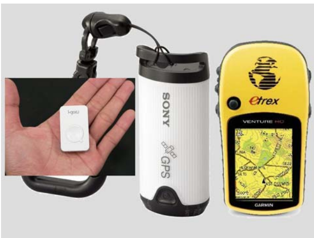
Figure 1: GPS logger I-GotU, Sony GPS-CS1 and the Garmin etrex mobile navigation unit
