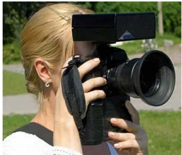
Figure 2: Telepointer GTA mounted on a SLR camera (image source www.gta-geo.de )
