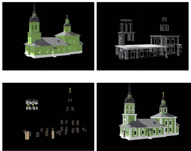
Figure 1: Structured VRML model. Top left: LOD 0, top mid-right: supplement to LOD 1, down left: supplement to LOD 2, down right: complete model containing all three sub-structures.
